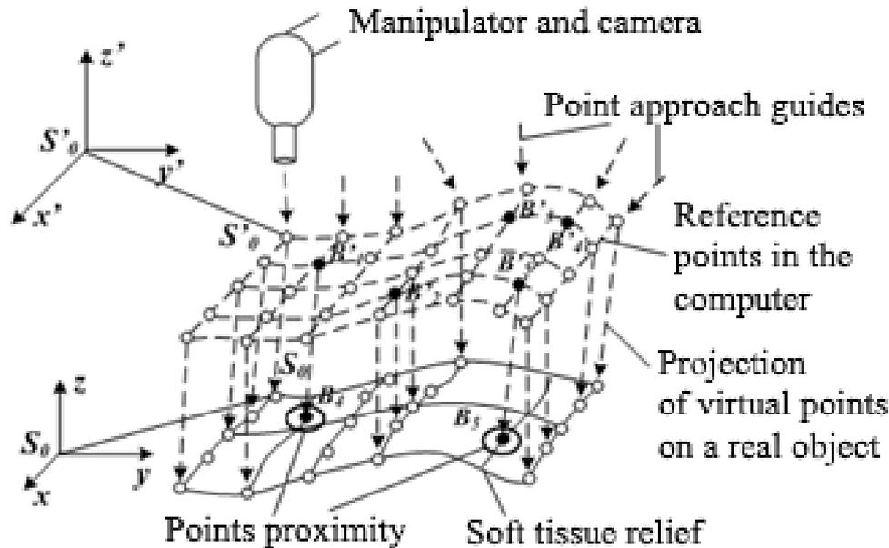
**Figure 1.** The scheme of transferring the virtual grid to the projected area.
