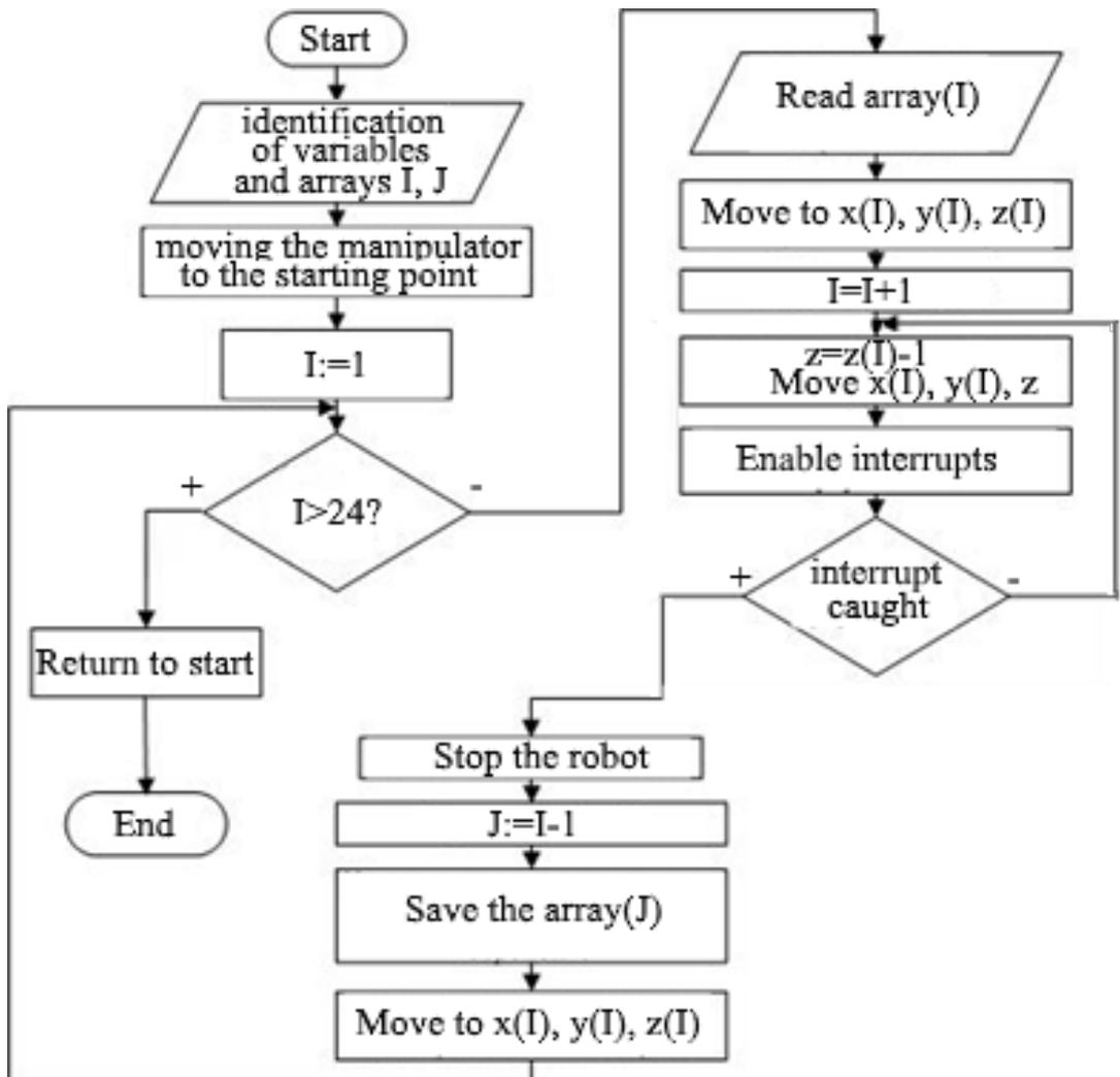
**Figure 2.** Block algorithm of the KR5 robot strength training implementation program for performing mechanical stimulation procedures.
